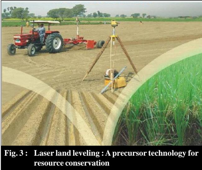
**Fig. 3 : Laser land leveling : A precursor technology for resource conservation**
